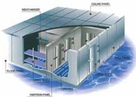
プレハブ冷蔵庫 Pre-fab ref. prov. chamber
