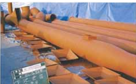
三菱重工業㈱向け集塵及び換気ダクト Dust collecting and ventilation duct for Mitsubishi Heavy Industries, Ltd
